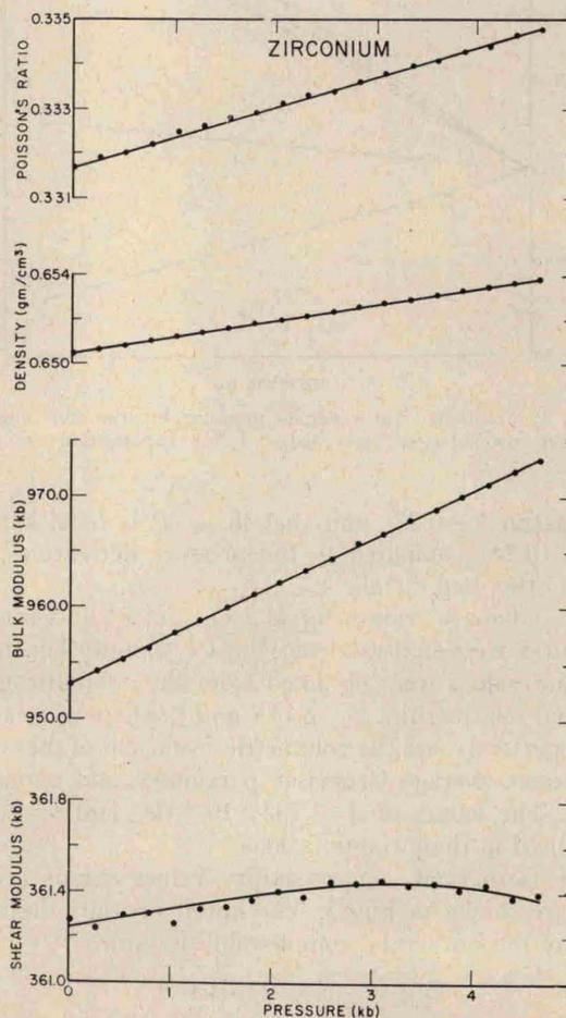
FIG. 4. Isotropic bulk and shear moduli, Poisson's ratio and density versus pressure.
